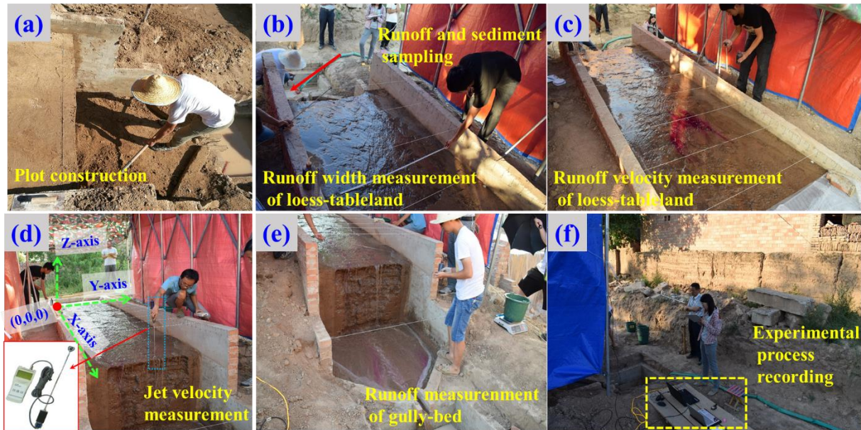
Figure 2 Runoff and sediment observation and recoding at upstream area, gully head and gully bed.
