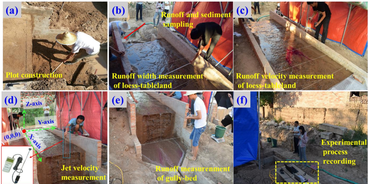
Fig. 3 Runoff and sediment observation and recoding at upstream area, gully head and gully bed.
