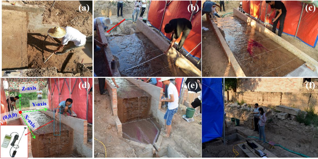
Figure 2. Plot construction (a), Runoff runoff width measurement of loess-tableland and runoff and sediment sampling of outlet (b) observation , runoff velocity measurement of loess-tableland (c), jet velocity measurement of gully head (d), runoff velocity and width measurement of gully bed (e), and experimental process recoding (f) at upstream area, gully head and gully bed.
