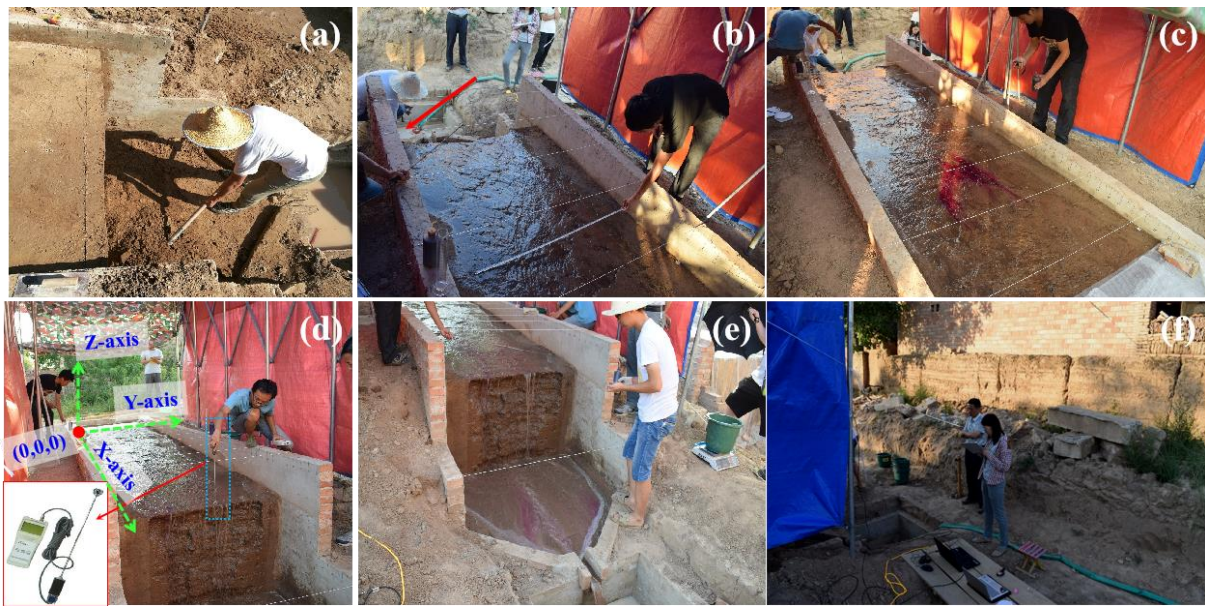
Figure 2. Plot construction (a), runoff width measurement of loess-tableland and runoff and sediment sampling of outlet (b), runoff velocity measurement of loess-tableland (c), jet velocity measurement of gully head (d), runoff velocity and width measurement of gully bed (e), and experimental process recoding (f)
