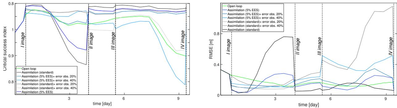
**Figure 12.** CSI values (on the left) and RMSE (on the right) after the standard assimilation of SAR observations free of errors (black), with 20% of errors (grey), with 40% of errors (light grey) and after the 5% EES assimilation free of errors (blue), with 20% of errors (light blue), with 40% of errors (cyan).
