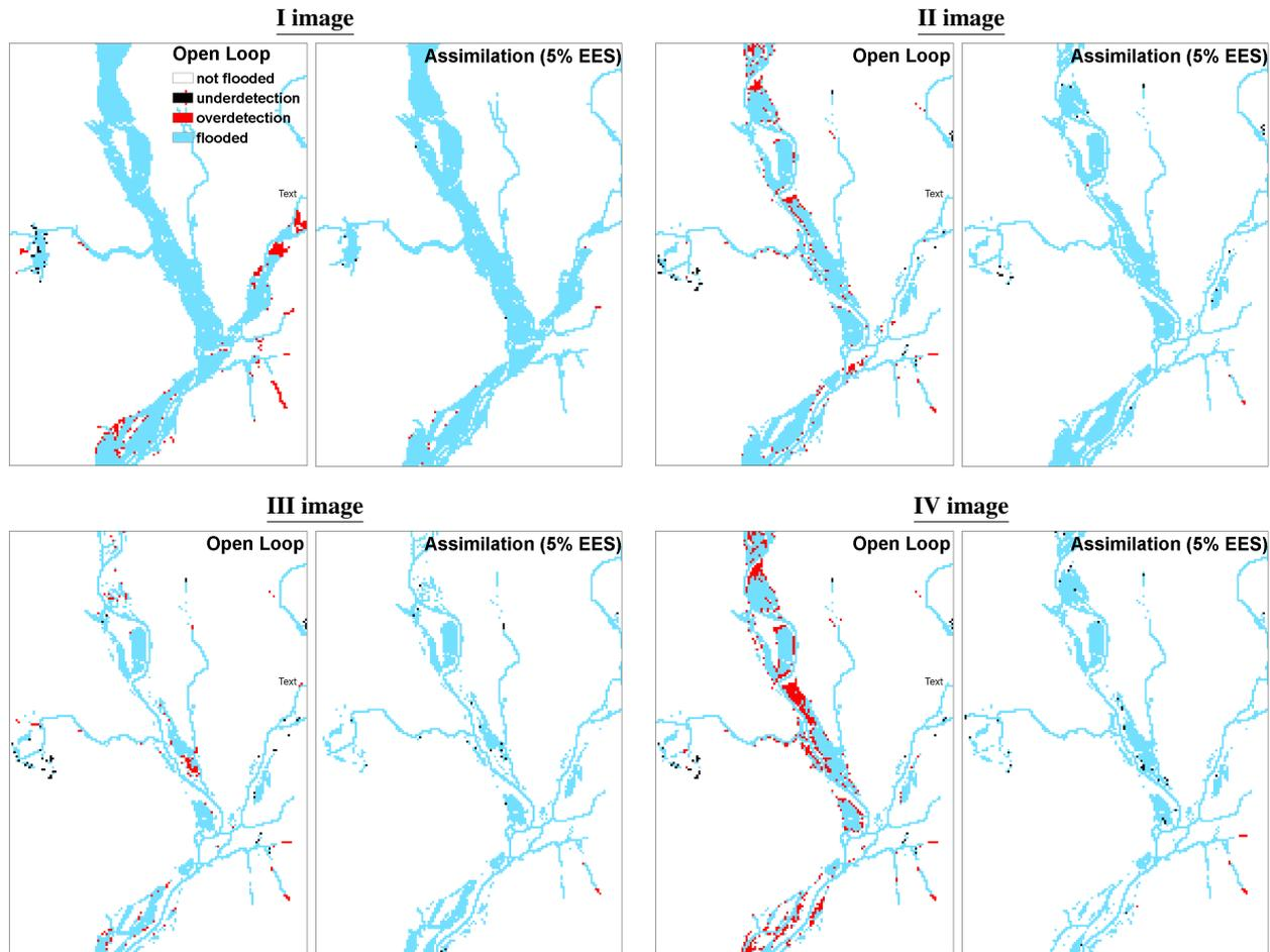
**Figure 7.** Contingency maps before (open loop) and after assimilation at 5 % EES at each time step. Two types of errors can be distinguished: over-detection (red pixels) when the model predicts the pixel as flooded but the pixel is observed as not-flooded and under-detection (black pixels) when the contrary occurs. In case model and observation agree pixels are correctly classified as not-flooded (white pixels) and flooded (blue pixels).
