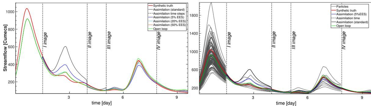
**Figure 11.** Streamflow time series at Bewdley. Left: assimilation runs with an EES of 5% (blue), 20% (cyan) and 50% (orange), OL (green), standard assimilation (black). Right: particles carrying significant weight after the assimilation at 5% EES (grey). Dashed lines correspond to the assimilation times.
