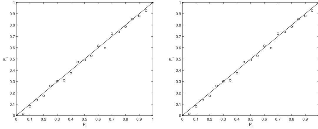
**Figure 5.** Example of the reliability plots for the verification of the synthetic probabilistic flood maps of the first two synthetic SAR images. On the x-axis probability range ( $P_i$ ), on the y-axis the fraction of pixels within the probability range of the probabilistic flood map observed as flooded in the *true* binary flood map ( $F_i$ ). The probabilistic flood maps are statistically reliable because the points align along the 1:1 line.
