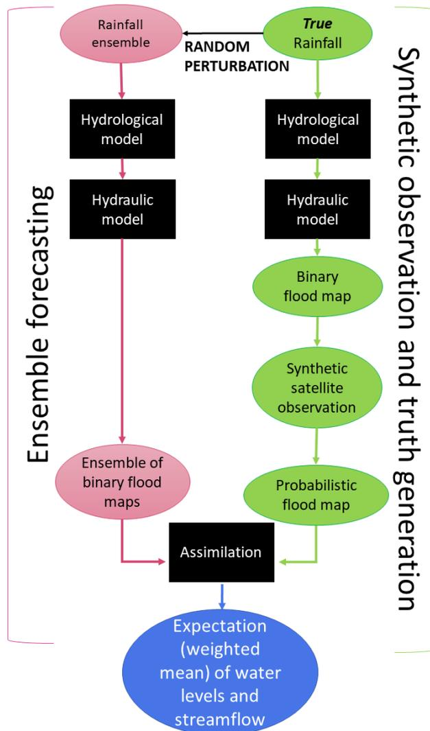
**Figure 1.** Flow chart of the synthetic experiment. The *true* rainfall is perturbed. The same flood forecasting model structure composed of a hydrologic model and a hydraulic model is used to obtain the probabilistic flood map and the ensemble of binary flood maps. The probabilistic flood map is assimilated into the ensemble of binary flood maps via the Particle Filter to obtain the weights with which the expectation of water levels, streamflow and flood extents are computed.
