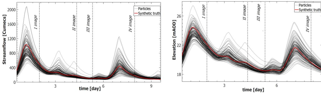
**Figure 6.** Streamflow time series (left) and water elevation time series (right) at the gauge station in Bewdley. Black lines represent the 128 particles while the red line corresponds to the synthetic truth.
