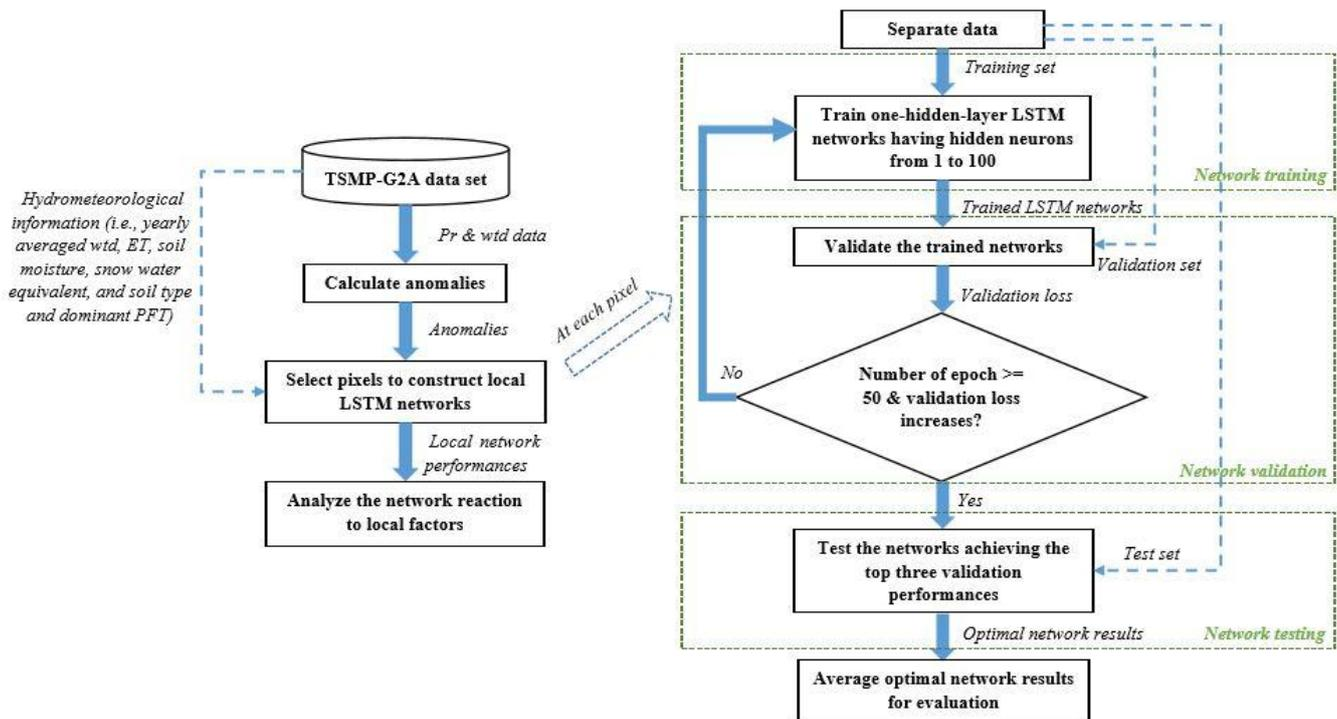
285 **Figure 4: Workflow for LSTM network setup over the European CORDEX domain. The left section represents the overall processes of the network setup, whereas the right section shows how to apply LSTM networks at a selected pixel. The dash lines with arrows indicate additional data transmission paths.**
