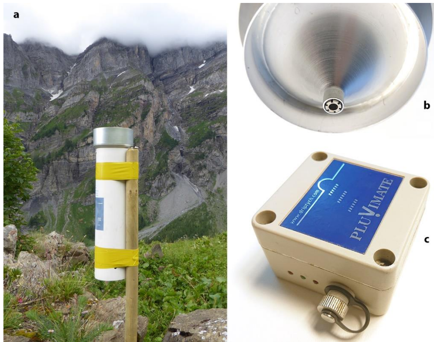
795 Figure 2. Drop-counting rain gauge used for rainfall measures. The Pluvimate is set-up vertically between 0.8 and 1.2 meters above the ground level (a). A tip at the end of the funnel (b) creates a calibrated drop of water that falls on the sensor, (c) which counts and records the number of drops during a given amount of time.
