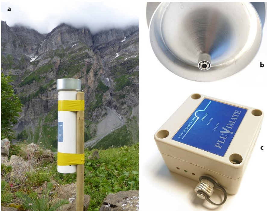
790 Figure 2. Drop-counting rain gauge used for rainfall measures. The Pluvimate is set-up vertically between 0.8 and 1.2 meters above the ground level (a). A tip at the end of the funnel (b) creates a calibrated drop of water that falls on the sensor, (c) which counts and records the number of drops during a given amount of time.
