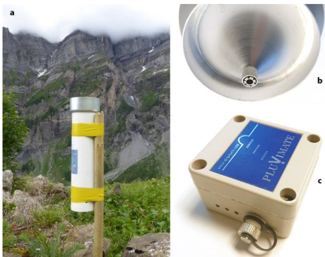
800 Figure 2. Drop-counting rain gauge used for rainfall measures. The Pluvimate is set-up vertically between 0.8 and 1.2 meters above the ground level (a). A tip at the end of the funnel (b) creates a calibrated drop of water that falls on the sensor, (c) which counts and records the number of drops during a given amount of time.
