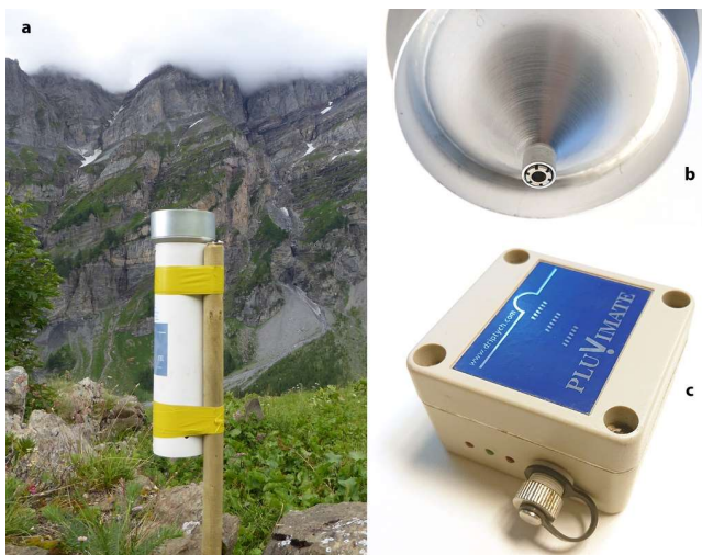
Figure 2.-Drop-counting rain gauge used for rainfall measures. The Pluvimate is set-up vertically between 0.8 and 1.2 meters above the ground level (a). A tip at the end of the funnel (b) creates a calibrated drop of water that falls on the sensor, (c) which counts and records the number of drops during a given amount of time.
