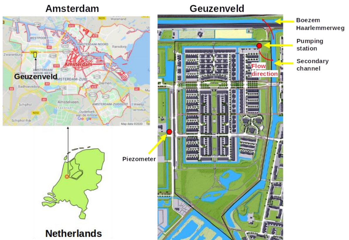
130 Figure 1 Location of polder Geuzenveld (source: © Google Maps ) and its landscape cross section and rain water and 131 groundwater drainage system
