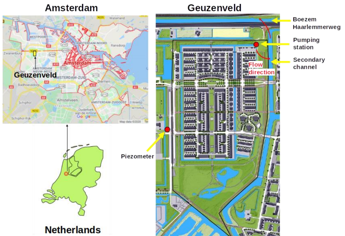
Figure 1 Location of polder Geuzenveld (source: © Google Maps ) and its landscape cross section and rain water and groundwater drainage system
