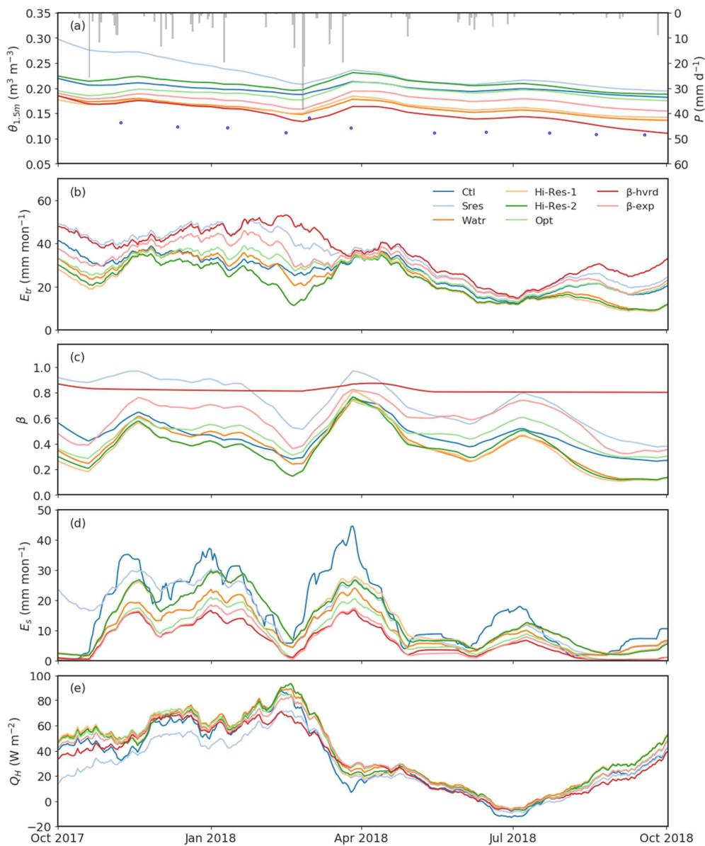
**Figure 8.** Simulations for each experiment during the drought period (October 2017 to September 2018). (a) the root zone soil moisture over top 1.5 m ( $\theta_{1.5m}$ ) and rainfall ( $P$ ; bars), with blue dots showing the observed soil moisture. (b)  $E_{tr}$ , (c) water stress factor ( $\beta$ ), (d)  $E_s$  and (e) sensible heat ( $Q_H$ ). All lines are smoothed with a 30-day window.
