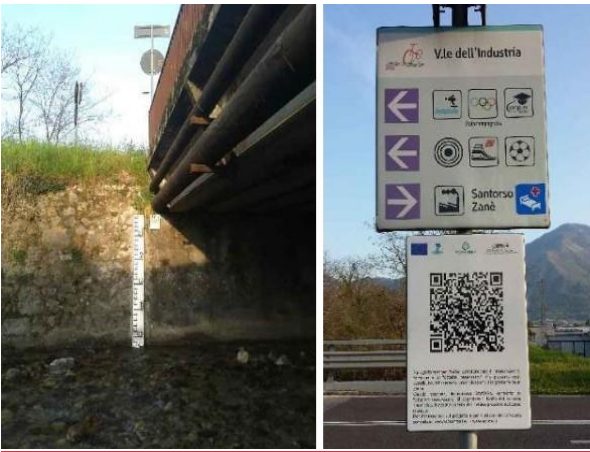
Figure 1: Photos showing staff gauges and QR codes used in the WeSenseIt project.
