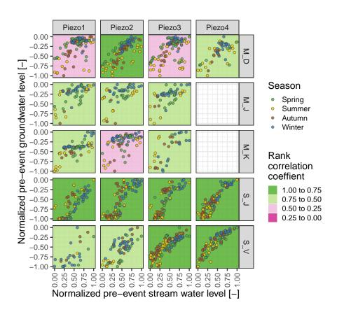
Figure 7. Normalised stream and groundwater levels before the investigated precipitation events ( $h_{preMin}$ ). The background colour represents the rank correlation coefficient, the point colours illustrate the season. Both axes are normalised by minimum and maximum  $h_{preMin}$  (see equation 1). The negative range on the y-axis indicates depths below ground (groundwater), the positive range on the x-axis depths above ground (stream).
