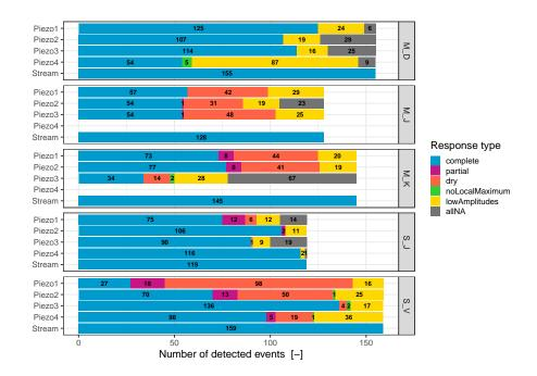
Figure 6. Number of detected events in the streams and groundwater at each stream gauge and piezometer, including types of event responses
