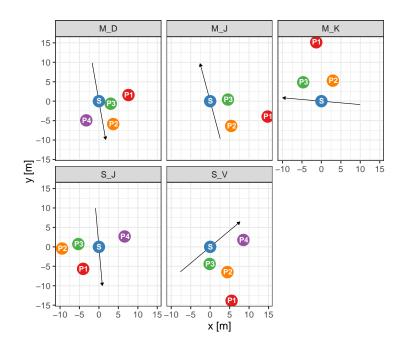
**Figure 2.** Schematic maps of the five sites. "P" stands for piezometer with the corresponding number while "S" stands for stream and is located at (0,0). The arrows point into the direction of stream flow. The coordinates are relative distances to the stream water level sensor (positive y-axis points north).
