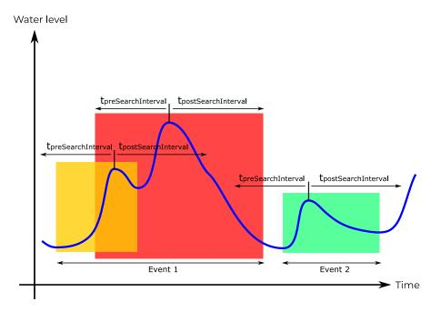
Figure 4. Merging conditions of consecutive events. Time series of water level showing three local maxima and the corresponding search windows for the minima. The coloured boxes mark the independently detected events as the interval between the two absolute minima around each peak within the respective search interval. The yellow and red events overlap and are merged into one. The green event is an independent second event.
