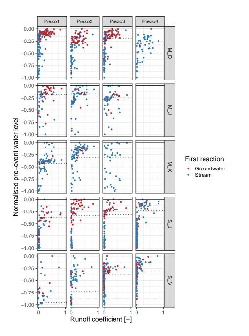
**Figure 10.** Event runoff coefficients versus shallow groundwater levels. Event runoff coefficients were determined for the Weierbach (schist) and Wollefsbach (marls) catchments where discharge data is available. The dotted horizontal lines illustrate the individual thresholds obtained from Figure 9. The point colours indicate whether the groundwater levels responded first (red) or the stream (blue).
