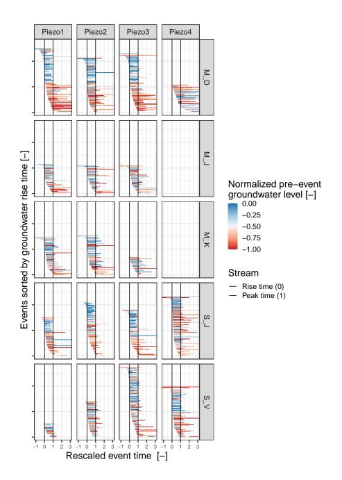
**Figure 8.** Timing of groundwater response relative to stream response. The two vertical lines at 0 and 1 represent the normalised rise and maximum time of each individual stream flow event. Horizontal bars each represent a groundwater event with its individual normalised rise and maximum time. Bluish colours indicate high and reddish colours indicate low pre-event groundwater levels.
