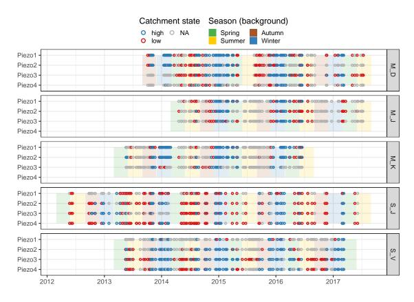
**Figure 11.** Catchment states at the beginning of events. In contrast to Figure 5 it shows whether or not the groundwater levels are above (high/blue) or below (low/red) the locally defined groundwater threshold levels. Only complete events are included, all other events are shown in grey (NA).
