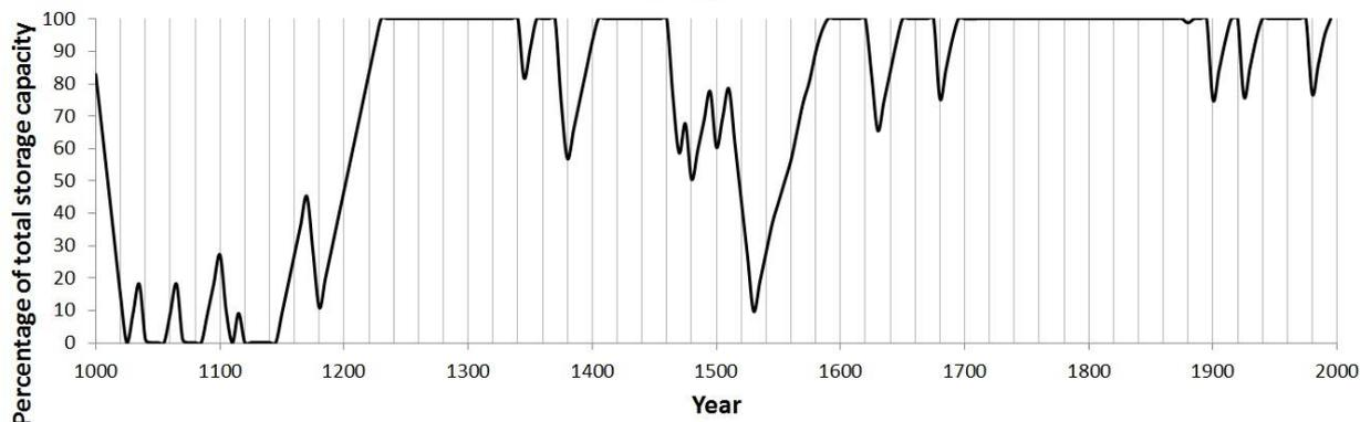
**Figure 8: Case study reservoir water storage levels based on initial storage in CE 1000 equal to 100% of capacity.**
