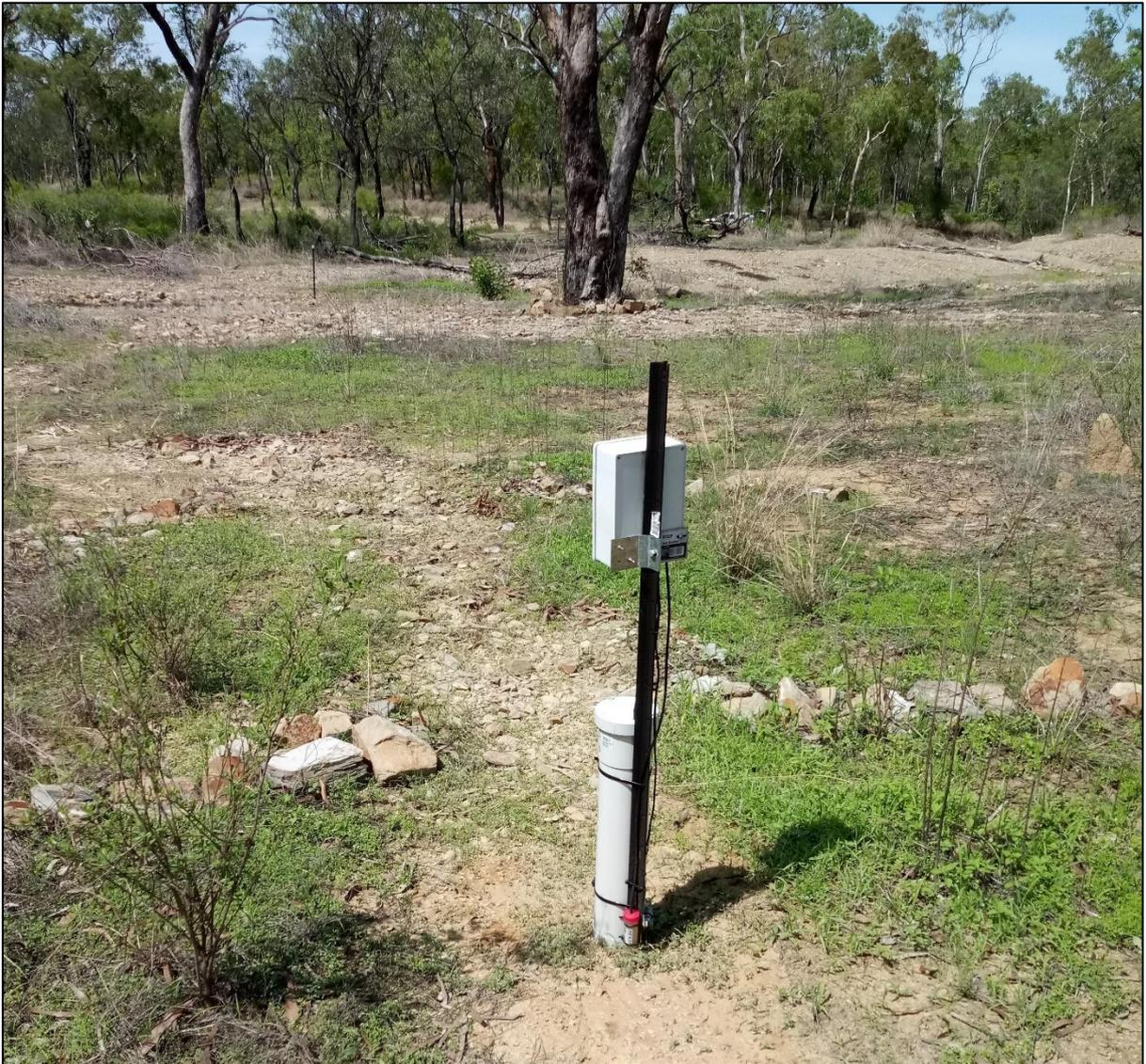
Figure SI-2 PASS sampler located in catchment drainage channel, upstream of the remediated gully.
