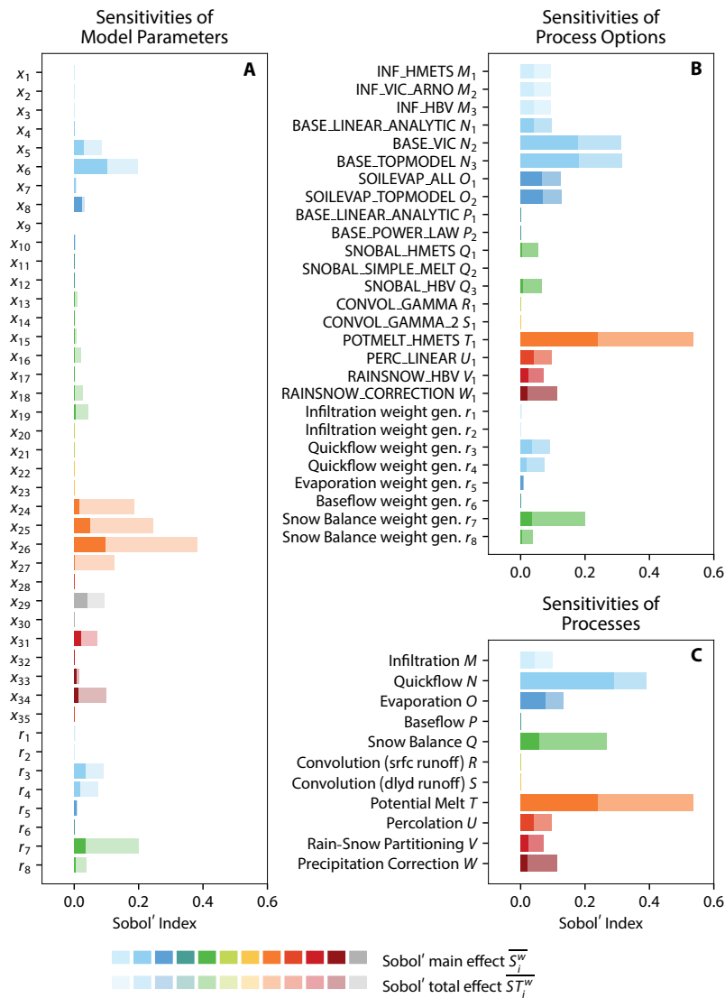
Figure 5. Results of the Sobol' sensitivity analysis of the hydrologic modeling framework Raven. (A) The sensitivities of 35 model parameters (see Table C2) and 8 parameters r_i that are used to determine the weights of process options are estimated. The Sobol' sensitivity index estimates are determined also for (B) 19 process options and (C) the 11 processes. The information which parameters are used in which process option and process can be found in Table C1. The different colors indicate the association of parameters and process options to the eleven processes. Parameters x_{29} and x_{30} are associated with several process options and are not colored but gray. The Sobol' main and total effects are shown (dark and light colored bars, respectively). All sensitivity index estimates shown are originally time-dependent and are aggregated as variance-weighted averages (Eq. 23 and 24). The average weights over the course of the year are shown in Figure 6.
