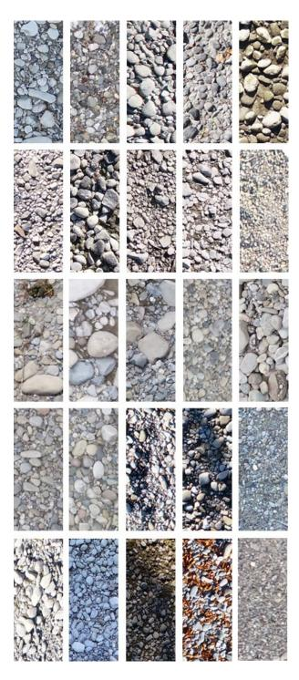
Figure 2. Example image tiles  $(1.25\,\text{m}\times0.5\,\text{m})$  with  $0.25\,\text{cm}$  ground sampling distance. Each of the 25 example tiles is taken from a different gravel bar.
