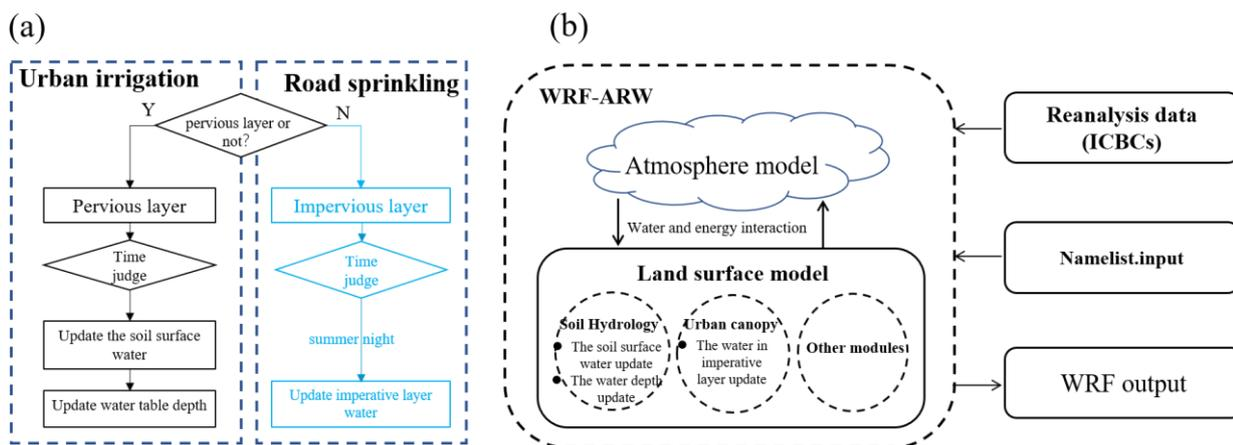
130 **Figure 1. Water usage scheme and its coupling with Weather Research and Forecasting (WRF) model. (a) Flow chart of water usage scheme including urban irrigation and road sprinkling, (b) schematic showing the Weather Research and Forecasting (WRF) model coupled with the water usage scheme.**
