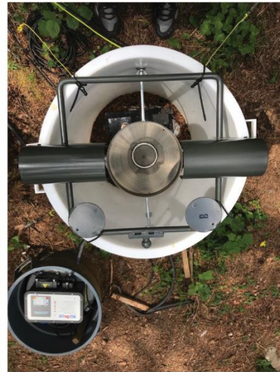
Figure 2. Setup for continuous measurement and sampling of open rainfall and throughfall. Diagram of the experimental equipment (left) and top view of the equipment installed in the forest stand (right).
