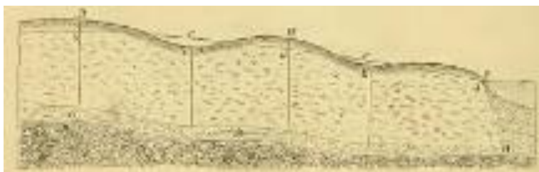
Fig. 9. Parabolic piezometric surface for a confined aquifer (Colding, 1872).
