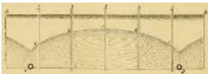
Fig. 10. Elliptic water table between drainpipes (Colding, 1872).
