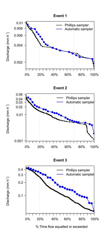
**Figure 5.** Flow duration curves covering the sampling period of the Phillips samplers. Blue line, samples taken with an automatic sampler for diatom analysis. Black line, continuous measurements of discharge at 15 min. intervals.
