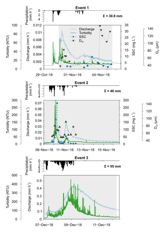
Figure 3. Catchment discharge, suspended sediment concentration (SSC), median particle size ( $D_{50}$ ), turbidity and precipitation for the three events. Discharge and turbidity were measured at 15 min. intervals, while SSC and  $D_{50}$  were analysed from automatic collected water samples. Total precipitation is given per event. Grey background gives the period the Phillips sampler was in the water.
