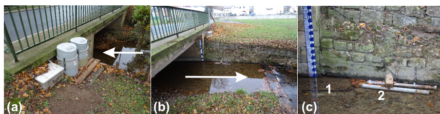
Figure 2. Pictures of the experimental set-up at the study location. (a), Automatic samplers installed upstream of the bridge. (b), Overview of the installation of the Phillips samplers. They were installed downstream of the bridge. The arrow denotes stream flow. (c), Close-up of the turbidity meter (1) and the Phillips samplers (2).
