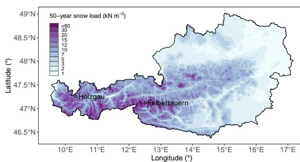
**Figure 7.** 50-year return levels of snow load in Austria. Two stations with *SWE* observations are outlined for a qualitative validation. This map bases on 214 snow height records,  $\Delta\text{SNOW.MODEL}$  derived *SWE*, and smooth spatial modeling of their extremes. See text for details.
