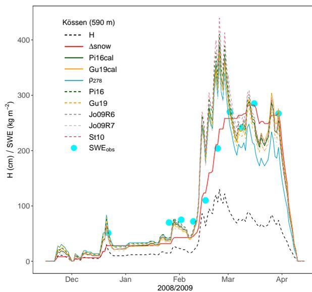
**Figure 6.** *SWE* simulations and observations (mostly weekly;  $SWE_{obs}$ ) for the winter 2008/09 in Kössen (cf. Fig. 5). Model abbreviations are given in the text and summarized in Fig. 4. See Table 2 for values, and consider the note in its caption. This plot is an illustration of the  $\Delta SNOW.MODEL$  performance during a distinct winter and outlines important features, which are addressed in the text.
