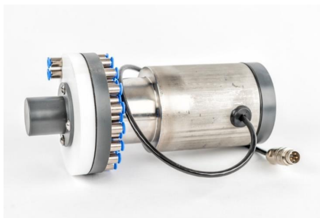
Figure 5 Assembled distribution unit (Photo by André Künzelmann, UFZ)
