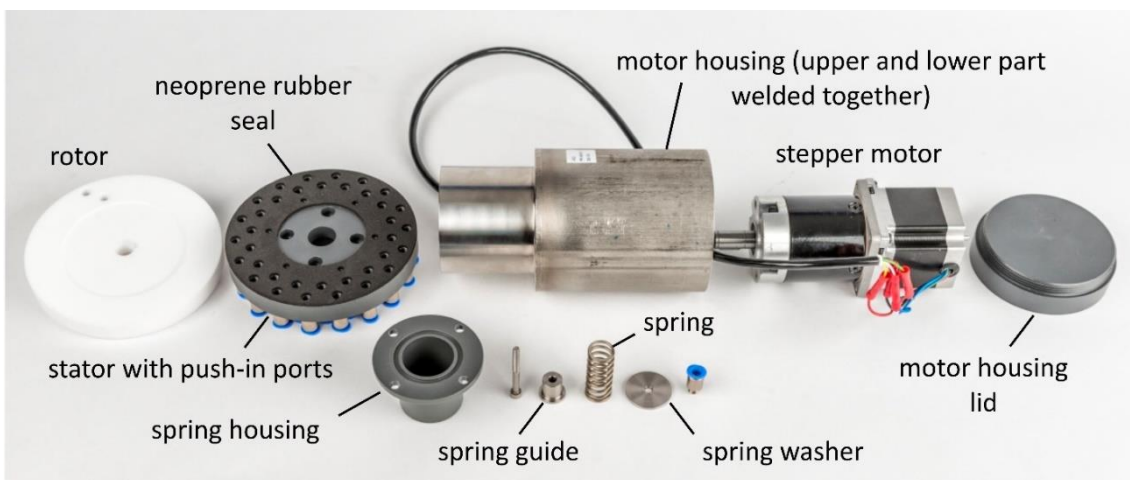
Figure 2 Overview of the main parts of the distribution unit (Photo by André Künzelmann, UFZ)
