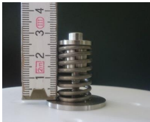
Figure 3 Spring for sealing pressure adjustment
