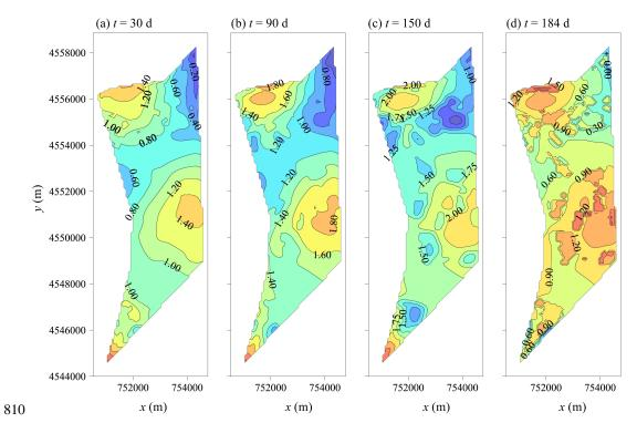
811 Fig. 10. Spatial simulated water table depth at different output times.
