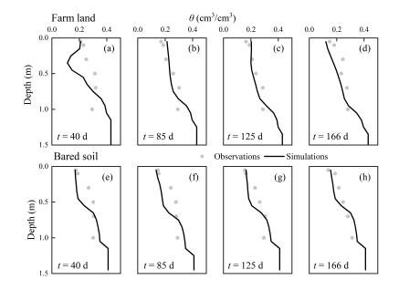
816 Fig. 11. Comparison between simulated and observed regional average soil water
