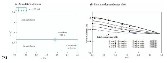
Fig. 4. (a) The sketch of the 2D recharge experiment. (b) The comparison of water table
