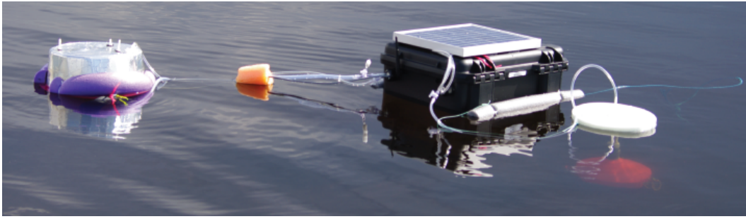
Figure 1: The photo of a deployed AFC_ABC device consists of a floating control box that houses the electronics, a floating chamber and a submerged funnel.
