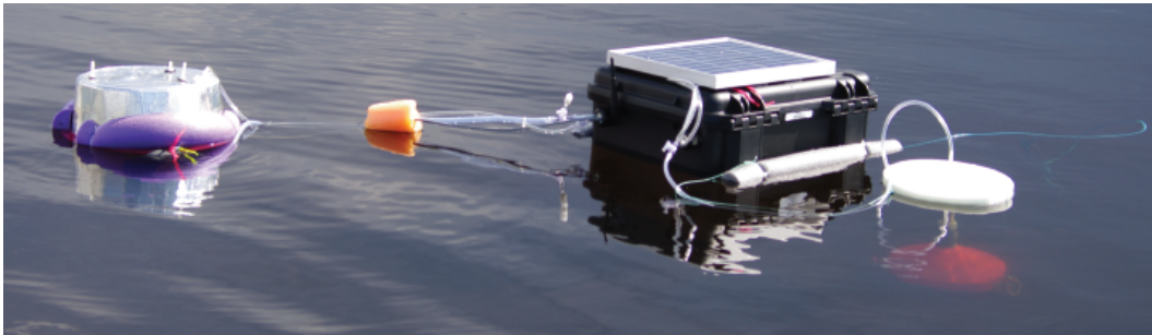
15 Figure 1: The photo of a deployed AFC_ABC device consists of a floating control box that houses the electronics, a floating chamber and a submerged funnel.
