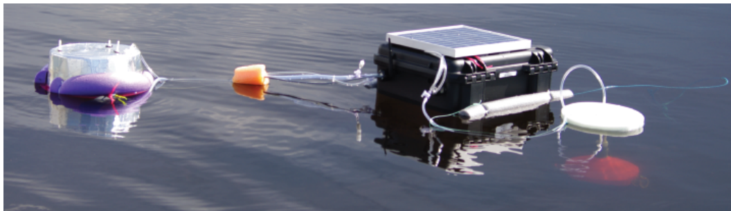
Figure 1: The photo of a deployed AFC_ABC device consists of a floating control box that houses the electronics, a floating chamber and a submerged funnel.
