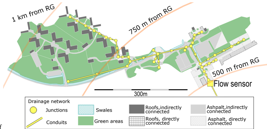
Figure 1. Map of the studied catchment showing elements of the high-resolution rainfall-runoff model (see Sect. 2.2) and the distance of the catchment to the rain gauge (RG). The diameters of the pipes range from 400 mm for the main trunk where the flow sensor is located to 200 mm for the smaller branches.
