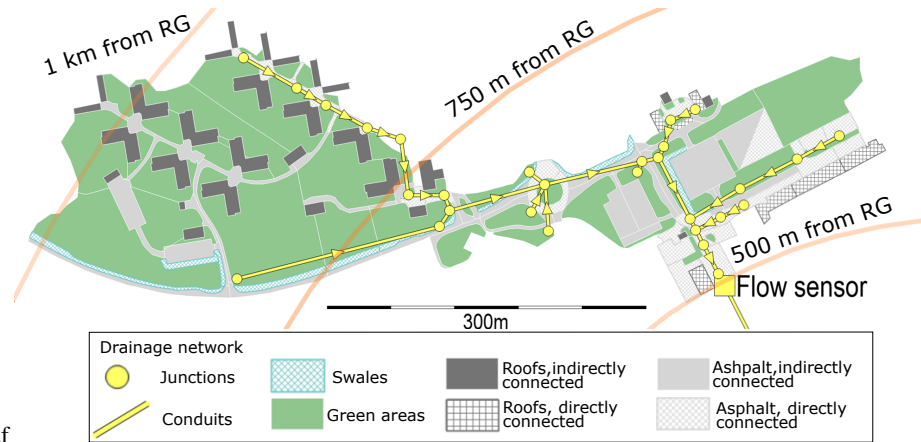
Figure 1. Map of the studied catchment showing elements of the high-resolution rainfall-runoff model and the distance of the catchment to the rain gauge (RG). The diameters of the pipes range from 400 mm for the main trunk where the flow sensor is located to 200 mm for the smaller branches.
