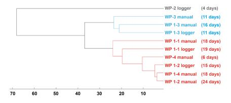
Figure 6. Results of cluster analysis of the drip site discharge time series, indicating the number of lag days calculated from the cross-correlation analysis. The gray cluster shows the drip site with the shortest lag to the antecedent rainfall (4 days), the blue cluster groups the drip sites with between 11 and 16 days lag to antecedent rainfall, and the red cluster includes drip sites with a lag to antecedent rainfall between 15 and 24 days, with the exception of WP-4 (see main text).
