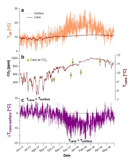
Figure 11. Comparison of meteorological parameters. a) daily mean air temperature at Waipuna station and in Waipuna Cave (in Organ Loft chamber). b) manual cave air CO<sub>2</sub> concentrations and daily mean air temperature in the Organ Loft chamber. c) calculated temperature difference ΔT between cave air and surface air from June to May 2018. During winter, the cave is warmer, and during summer, the cave is colder compared to the surface air.
