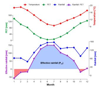
Figure 4. Mean monthly temperature (red line), precipitation (blue line), and Priestley-Taylor potential evapotranspiration (PET) recorded at Te Kuiti Ews station between 2002 and 2019 (green line) (http://cliflo.niwa.co.nz), and difference between rainfall and PET (purple line). The shaded blue area represents the effective rainfall ( $P_{\rm eff}$ ).
