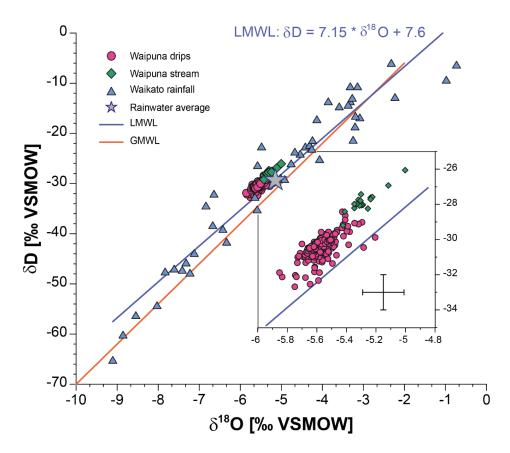
Figure 7. Cross-plot of  $\delta D$  versus  $\delta^{18}O$  in dripwater (pink circles), the Waikato region precipitation (blue triangles) and Waipuna stream (green diamonds). All cave waters fall in a very narrow range (inset) and within error on the Local Meteoric Water Line (blue line, Keller et al., 2014). The cross in the inset shows the  $2\sigma$  uncertainties for  $\delta^{18}O$  and  $\delta D$ .
