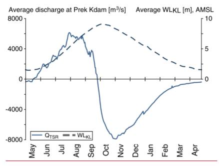
Figure 5. Daily averaged (from 1997 to 2004) water discharge hydrograph at Prek KDam and water level variation at Kampong Luong (Kummu et al., 2014). The solid line presents river flow coming in the Tonle Sap Lake at the Prek Kdam station, while the dashed line shows water levels at Kampong Luong station.
