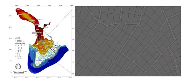
Figure 4. The modelling grid. The floodplains are defined as 2D grids (in black) and canals are defined as 1D networks (in pink). The connecting links of 1D network and 2D grids are in blue.
