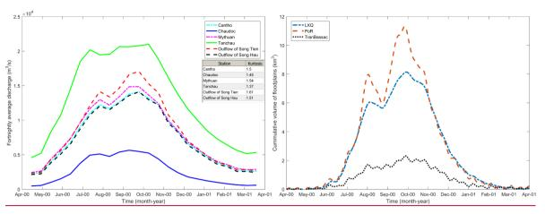
Figure 10. Fortnightly average discharges at stations along the Mekong branches (left) and cumulative water volumes of the major floodplains in the VMD (right).
