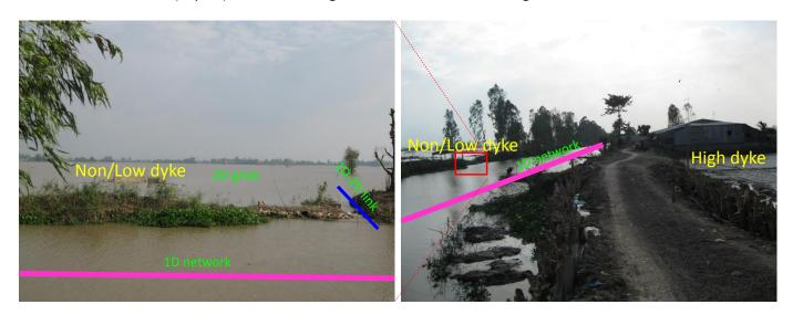
Figure 5. A high dyke and non/low dyke in An Giang province and their schematization in modelling. Photos by Vo Quoc Thanh 2012.
