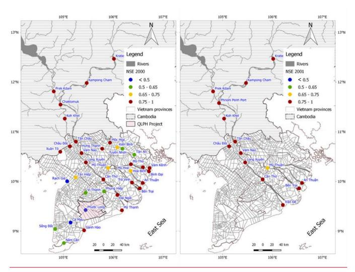
Figure A1. NSE values of water levels at the gauging stations in the Mekong Delta. The calibration (the year 2000) and validation (the year 2001) are presented on the left and right maps respectively.
