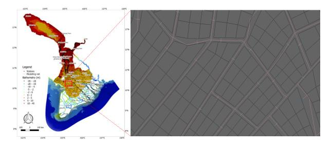
Figure 2. The modelling grid. The floodplains are defined as 2D grids (in black) and canals are defined as 1D networks (in pink). The connecting links of 1D network and 2D grids are in blue.
