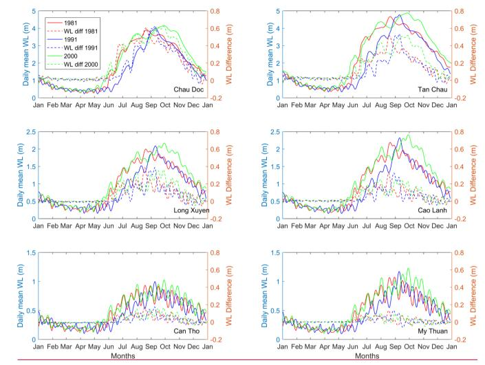
Figure 13. Simulated daily mean water levels in high-flood years of 1981, 1991 and 2000 at selected stations on the Mekong River. The dashed lines indicate water level differences due to impacts of high dykes.
