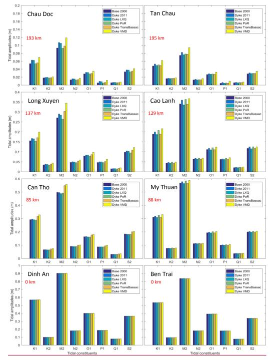
Figure 12. Tidal amplitudes of the 8 main constituents at the selected stations along the Song Tien (right) and Song Hau (left) from the river mouths to about 195 km landward in the scenarios of high dyke development.
