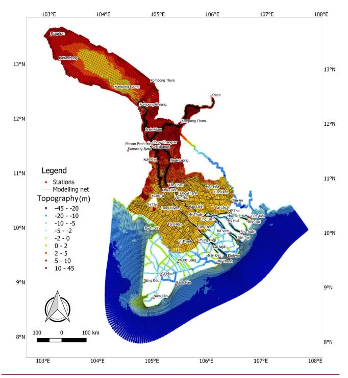
Figure 6. Mekong Delta modelling grid and River river bathymetry interpolated topography from 1D ISIS cross-section data interpolation and shelf bathymetry topography of the Mekong Delta.
