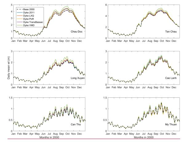
Figure 11. Daily mean water level variations at selected stations along the Song Hau (left) and Song Tien (right) under different scenarios of high dyke development.
