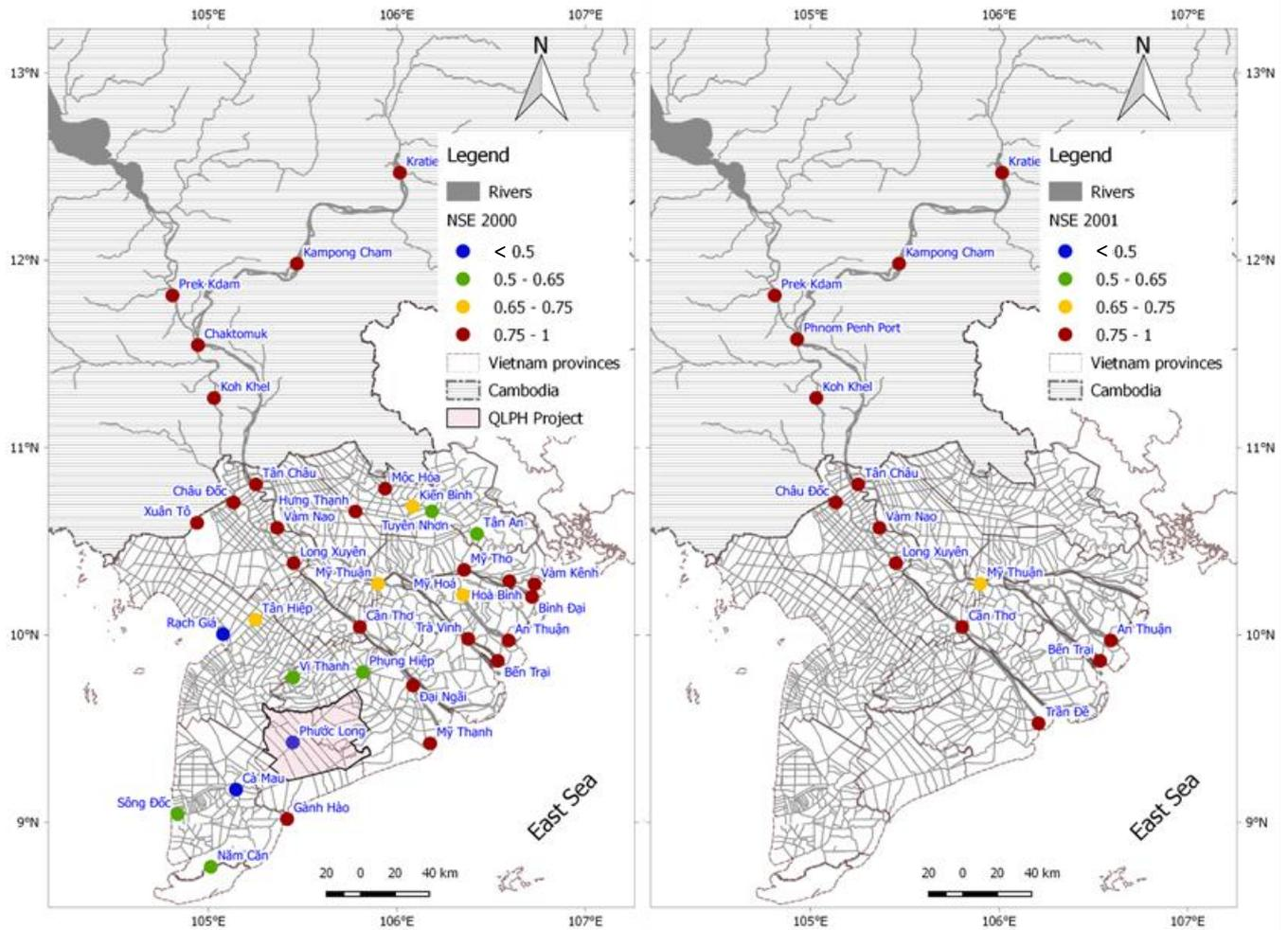
**Figure A1. NSE values of water levels at the gauging stations in the Mekong Delta. The calibration (the year 2000) and validation (the year 2001) are presented on the left and right maps respectively.**
