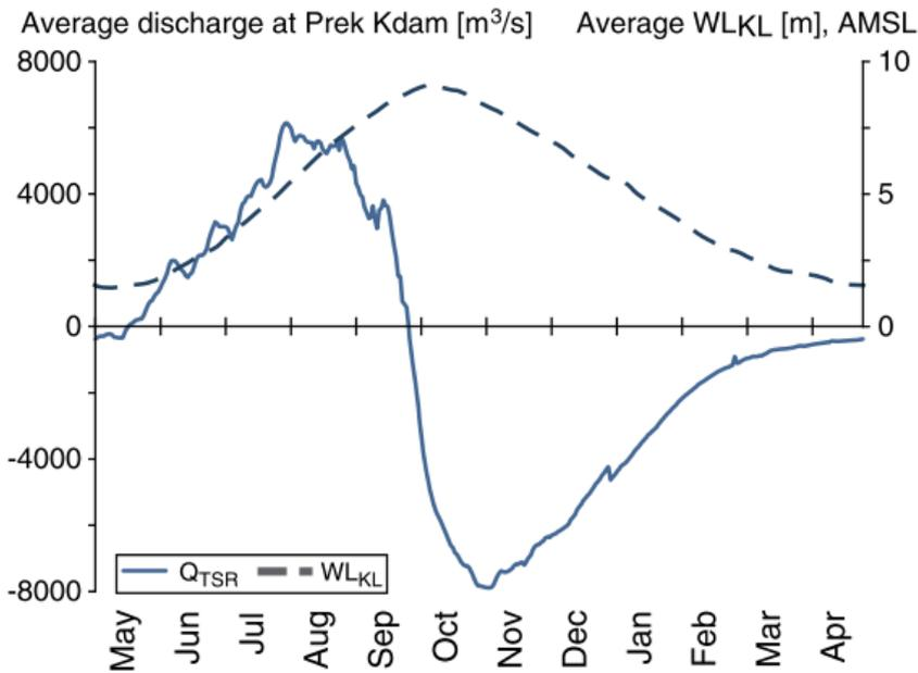
**Figure 5. Daily averaged (from 1997 to 2004) water discharge hydrograph at Prek Kdam and water level variation at Kampong Luong (Kummu et al., 2014). The solid line presents river flow coming in the Tonle Sap Lake at the Prek Kdam station, while the dashed line shows water levels at Kampong Luong station.**
