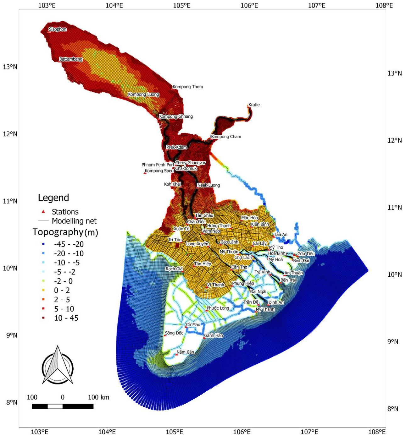
**Figure 6. Mekong Delta modelling grid and River-river bathymetry-interpolated topography from 1D ISIS cross-section data-interpolation and shelf bathymetry-topography of the Mekong Delta.**
