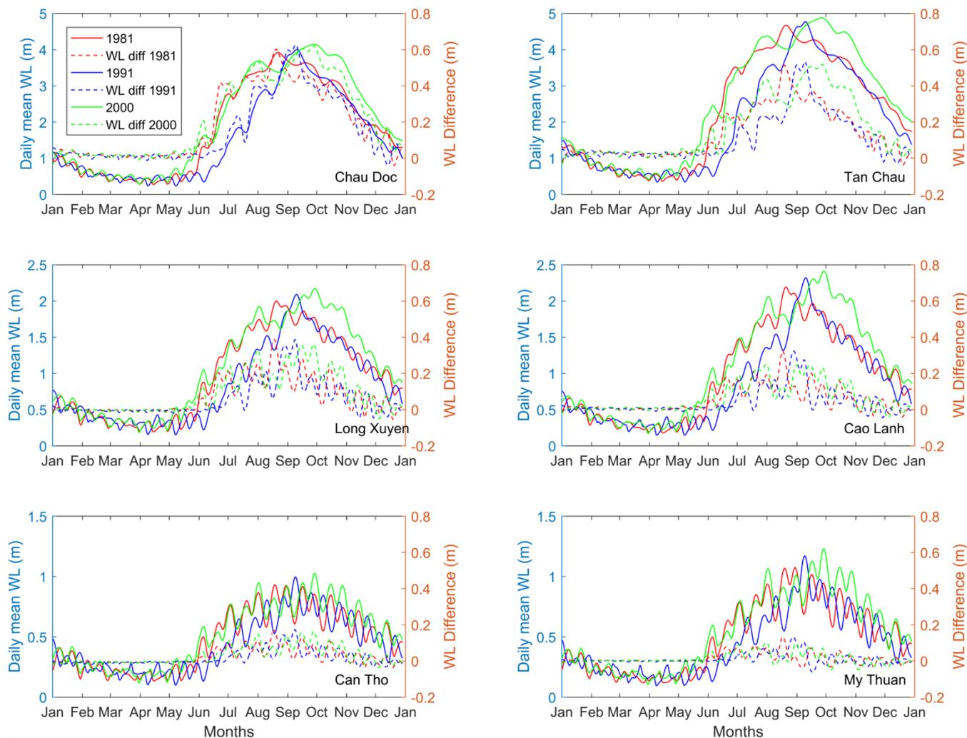
**Figure 13. Simulated daily mean water levels in high-flood years of 1981, 1991 and 2000 at selected stations on the Mekong River. The dashed lines indicate water level differences due to impacts of high dykes.**
