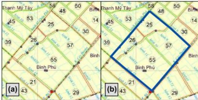
Figure 1. An example of high dykes and low dykes; (a) high dykes in orange and low dykes in green; (b) the blue line presents a low dykes in modelling. (After Triet et al. 2017)
