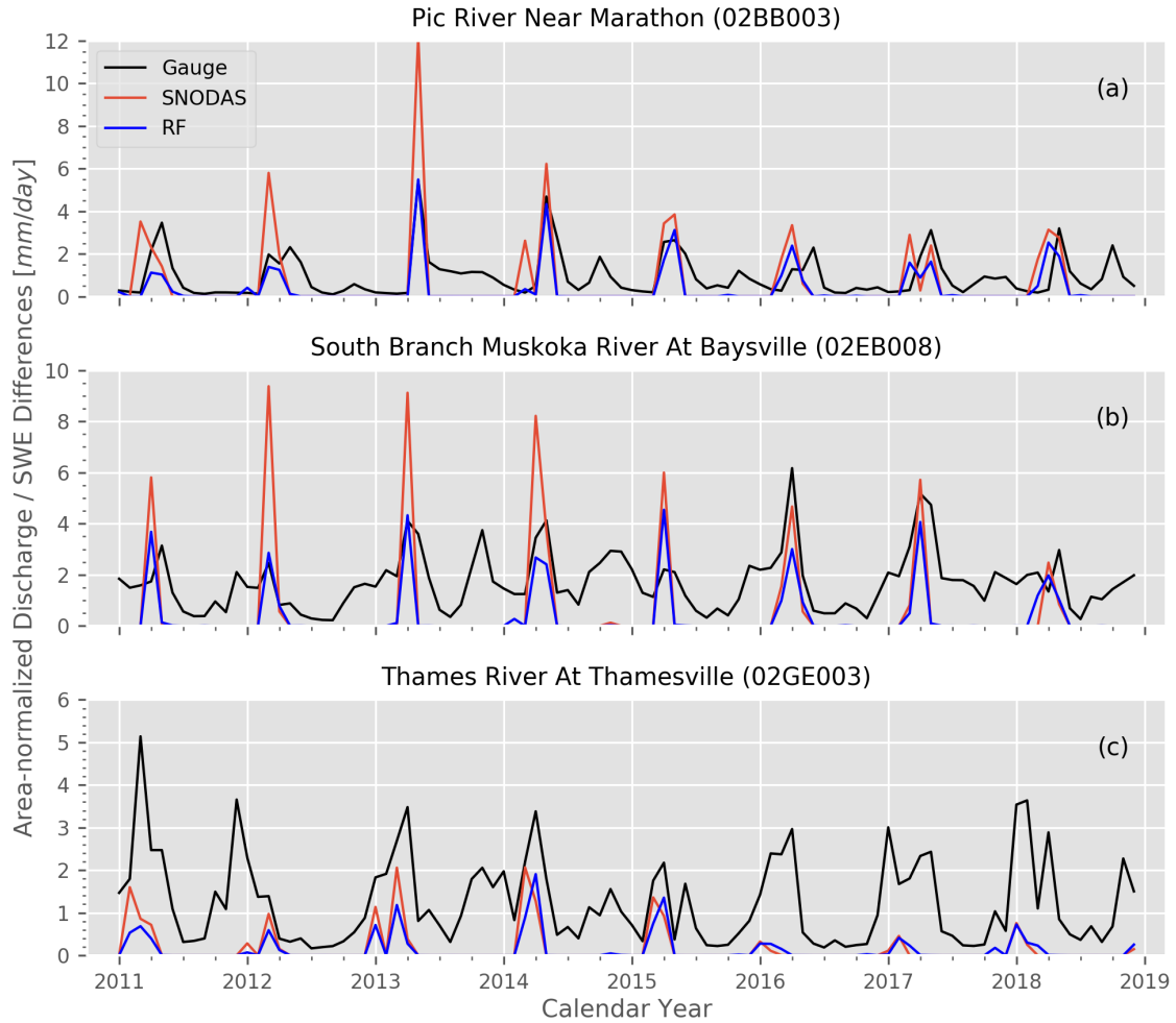
Figure 7. Monthly timeseries of area-normalized discharge from three river gauges in Ontario, along with corresponding melt estimates calculated from the SNODAS and RF corrected SWE datasets. Melt estimates are negative monthly SWE differences averaged over the drainage area of the corresponding gauge (see section 4.1).
