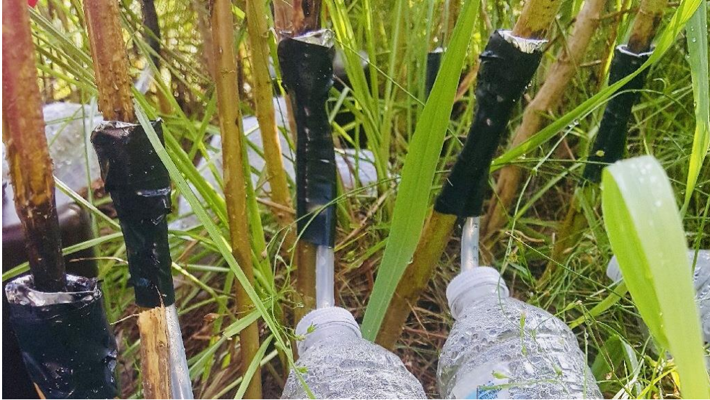
Figure S3. Photograph of the dogfennel stemflow collars.
