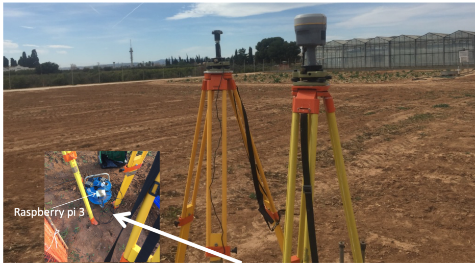
Figure 3. Instrumental configuration in the field campaign. A geodetic-quality GNSS antenna and a mass-market GNSS antenna were working at the same time.
