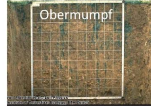
Figure 3 Finger flow pattern revealed from standardized dye staining experiments for a transport time of 1 day; images were generously provided by Flury et al. (2004; 2005; Copyright © 1994, 1995 the American Geophysical Union) for Switzerland, Blume et al. (2009, Copyright © Theresa Blume) for Chile, Wienhöfer et al. (2009, Copyright © Jan Wienhöfer KIT) for Austria, and Zehe and Flüher (2001, Copyright © Erwin Zehe KIT) and van Schaik et al. (2014, Copyright © 2013 John Wiley & Sons, Ltd.) for the German Weierbach.
