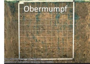
Figure 3 Finger flow pattern revealed from standardized dye staining experiments for a transport time of 1 day; images were generously provided by Flury et al. (2004; 2005; Copyright © 1994, 1995 the American Geophysical Union) for Switzerland, Blume et al. (2009, Copyright © Theresa Blume) for Chile, Wienhöfer et al. (2009, Copyright © Jan Wienhöfer KIT) for Austria, and Zehe and Flühler (2001, Copyright © Erwin Zehe KIT) and van Schaik et al. (2014, Copyright © 2013 John Wiley & Sons, Ltd.) for the German Weiherbach.
