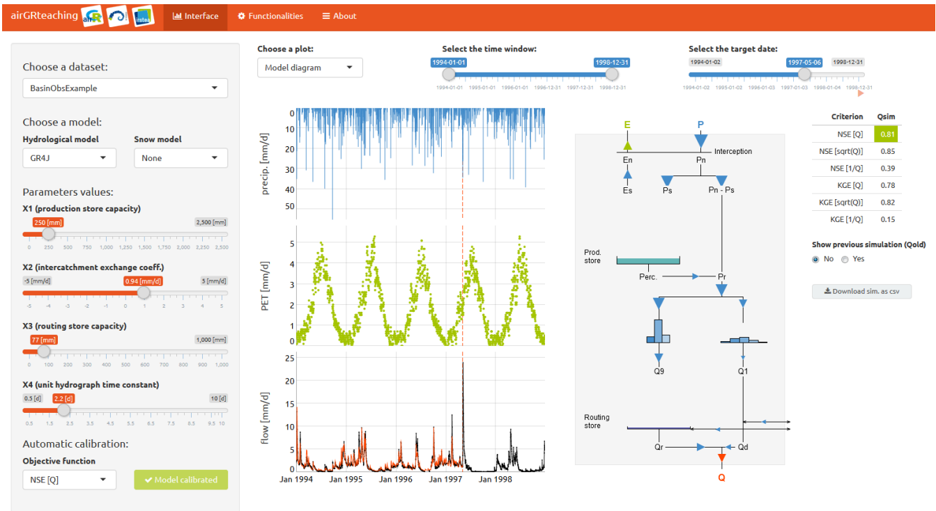
Figure 6. The airGRteaching interface that is used for teaching hydrological modelling. Students can choose a catchment dataset, a hydrological model and activate a snow model on the top left panel of the interface. Modifying the parameters values (on the left) by using the sliding bars will automatically update the graphs and scores displayed (on the right). This interface highlights in an interactive manner the basic principle of the rainfall-runoff relationship and its description in hydrological models. On the bottom left of the interface, an objective function can be chosen and an automatic calibration procedure can be launched within the interface.
