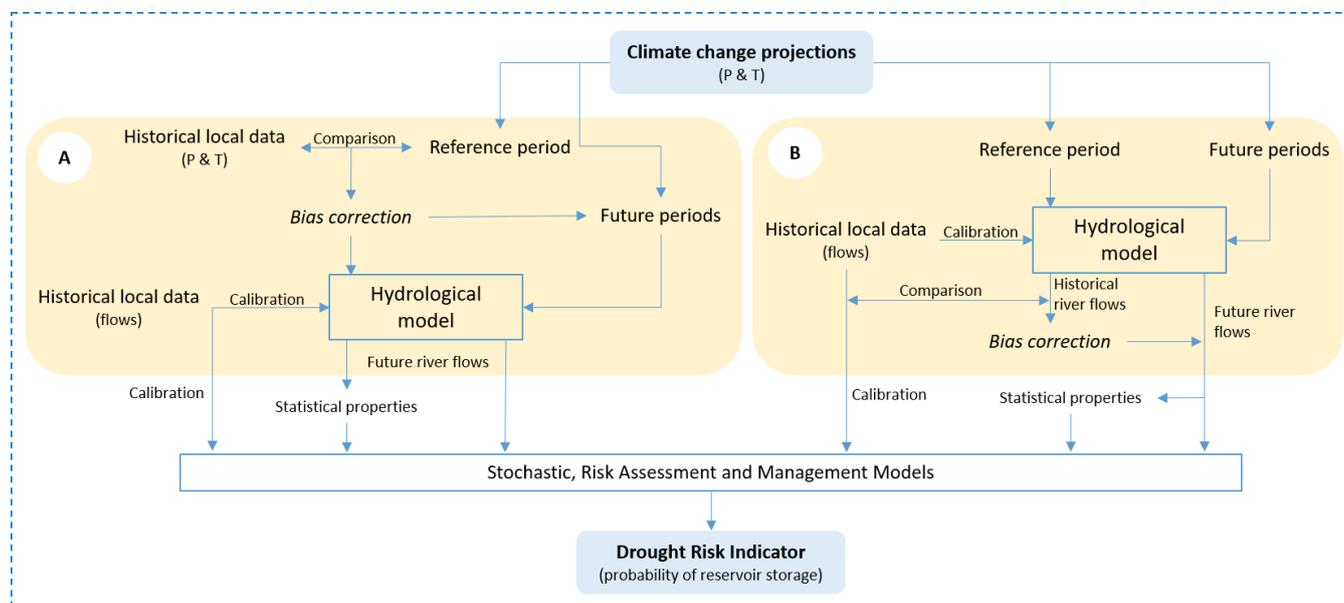
145 **Figure 3. Detailed workflow for characterising natural flows using a bias correction before (A) and after (B) the hydrological model.**
