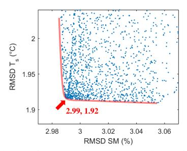
**Figure 4**. Objective function values of evaluated parameter sets and corresponding Pareto front. The x-axis is the objective function for simulating SM. The y-axis is the objective function for simulating  $T_s$ . Each dot corresponds to one simulation
