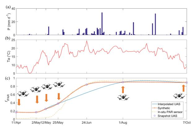
**Figure 2**. (a) Daily precipitation (P, mm·d<sup>-1</sup>), (b) Daily air temperature (T<sub>a</sub>, °C), and (c) Daily fraction of the intercepted PAR ( $f_{IPAR}$ ) interpolated from UAS based NDVI during the growing season of 2016.
