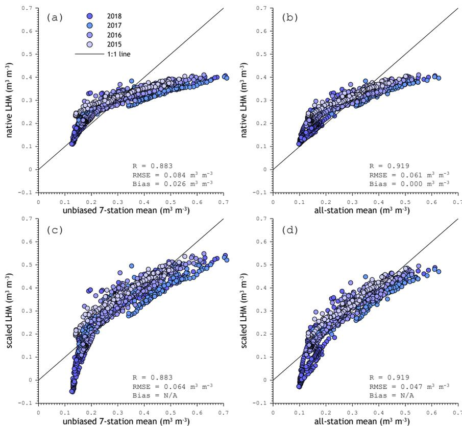
**Figure 6.** LHM simulated spatial mean soil moisture against references deduced from *in situ* measurements for SMAP reference pixel 4371; a) and b) show the native LHM simulations versus the unbiased 7-station mean and all-station mean, respectively; c) and d) presented the same as a) and b) only LHM soil moisture is scaled to the statistical moments (1<sup>st</sup> and 2<sup>nd</sup>) of the *in situ* references.
