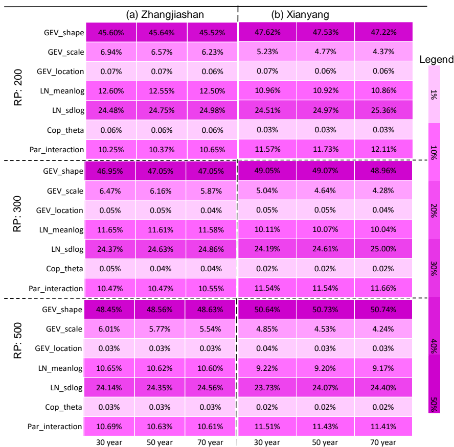
Figure 11. Contributions of parameter uncertainties to predictive failure probabilities in OR under different design standards (i.e. return periods (RP)) and different service periods
