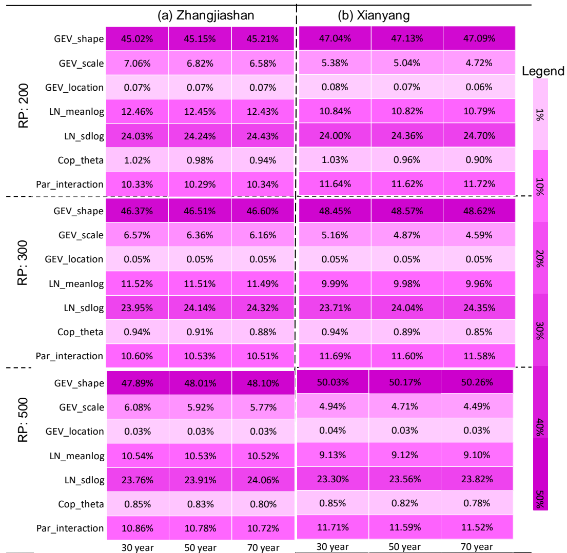
Figure 12. Contributions of parameter uncertainties to predictive failure probabilities in Kendall under different design standards (i.e. return periods (RP)) and different service periods
