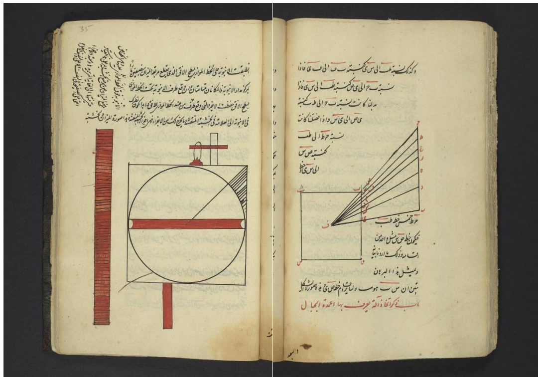
Figure 6. Illustration for the proof on how to vertically to describe how to measure and determine the height of a mountain. Diagrams f35r and f36v from Karaji (1675). Permanent Link: http://hdl.library.upenn.edu/1017/d/medren/9948256513503681
