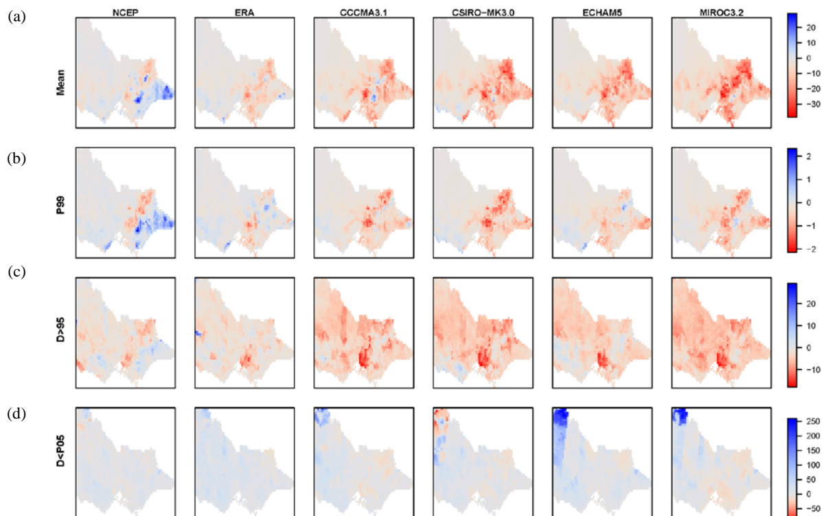
Figure 3 Historical (1990-2009) runoff simulation bias (i.e. runoff using WRF-BC rainfall minus using AWAP rainfall) for (a) mean annual runoff (mm), (b) daily 99 th percentile runoff (mm), (c) number of days exceeding AWAP 95 th percentile, (d) number of days below AWAP 10 th percentile. Panels (left to right) are using WRF-BC rainfall forced by two reanalysis (NRR, ERAI) and then four GCMs (CCCMA3.1, CSIRO-MK3.0, ECHAM5 and MIROC3.2).
