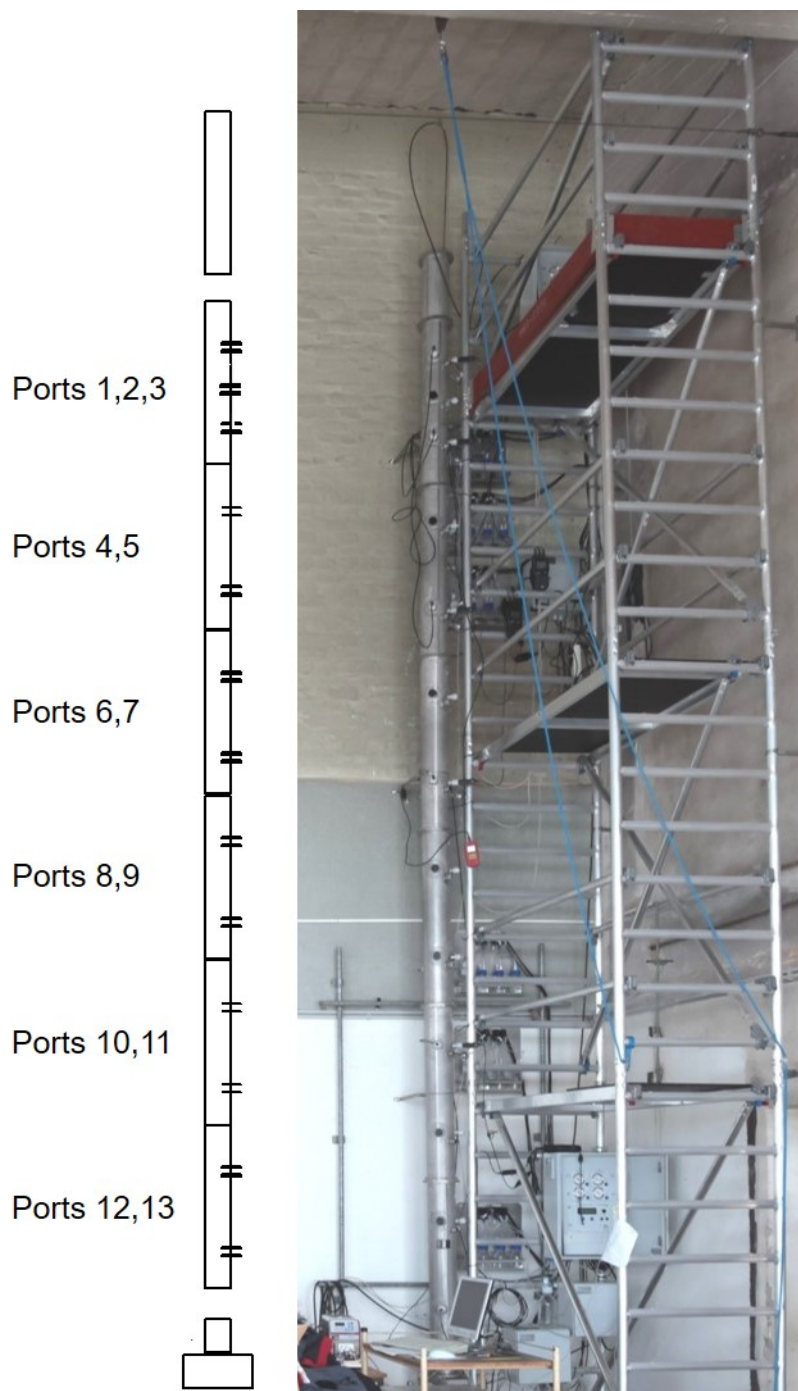
Figure 1. The six-meter long column, Dresden, Germany. Sensors were located in ports 1, 3, 5, 7, 9 and 13
