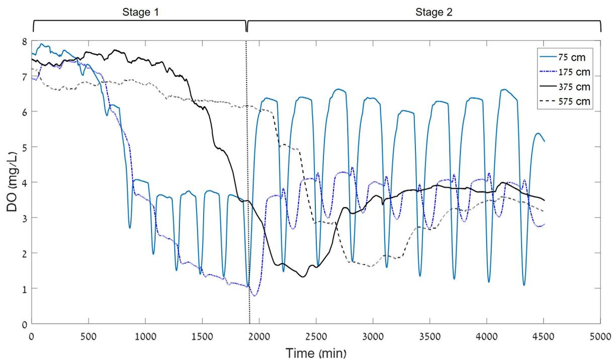
**Figure 3.** DO concentrations at depths of 75, 175, 275 and 575 cm in response to the increase in DP (between SW150 and SW240). Note the convergence of the deep sensors to  $< 2$  mg/l during the short DP versus convergence to  $> 3$  mg/l in response to the longer DP.
